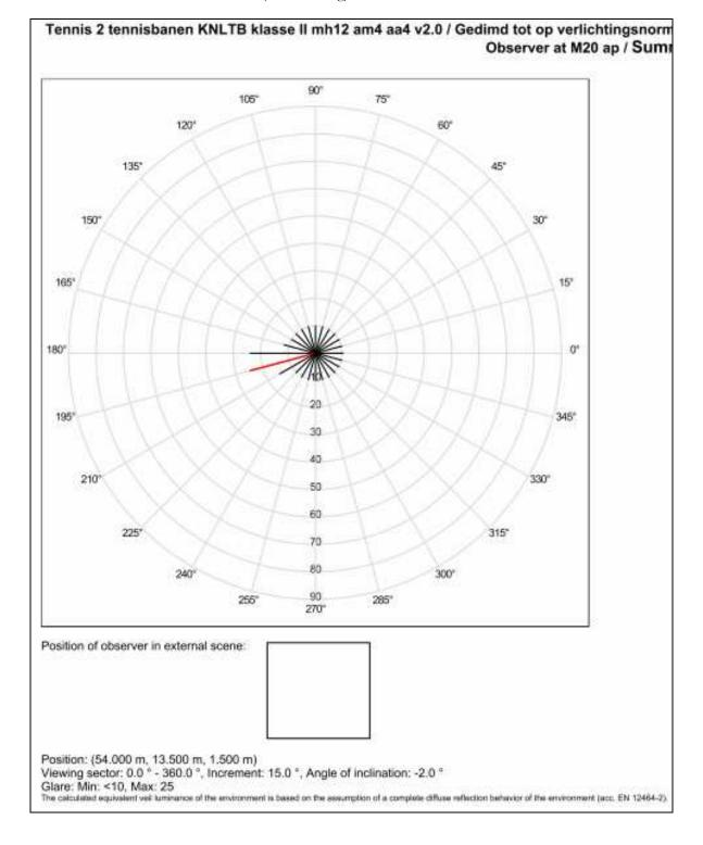
The illustration below shows the GR (Glare Rating) for an observer on the A420:
